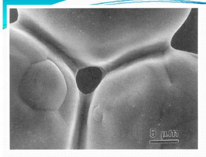
Spherical particle  $\rightarrow$  convex surface  $\rightarrow$  mass source Pore  $\rightarrow$  concave surface  $\rightarrow$  mass sink
