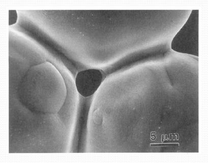
A reduction in interfacial energy  $(\Delta y)$  takes place by the replacement of solid/vapour interfaces by solid/solid interfaces.
