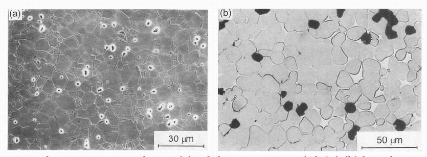
Typical microstructures during (a) solid state sintering (Al<sub>2</sub>O<sub>3</sub>) (b) liquid phase sintering (98W-1Ni-1Fe(wt%))
